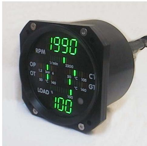
The Display receives CAN-Bus-Messages from the ECU to be displayed. There are RPM, Load, oil pressure, oil temperature, cooling fluid temperature and gearbox temperature. Furthermore, the display is capable of warning the pilot if one of these values is out of the green range. In this case, the Master Caution Lamp is activated. The Master Caution Lamp is only activated if the caution condition is steady for at least these times in order to suppress short intermittent conditions:
